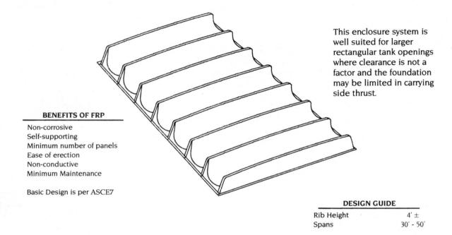
FRP is most advantageous in meeting structural requirements in hostile environments. SynTechnics free-spanning scalloped flat covers are structurally designed to handle appropriate live, wind, and unbalanced loading conditions. Various accessories such as windows, duct connections, vents, personnel doors and equipment hatches are readily available, sized to meet operating conditions.
